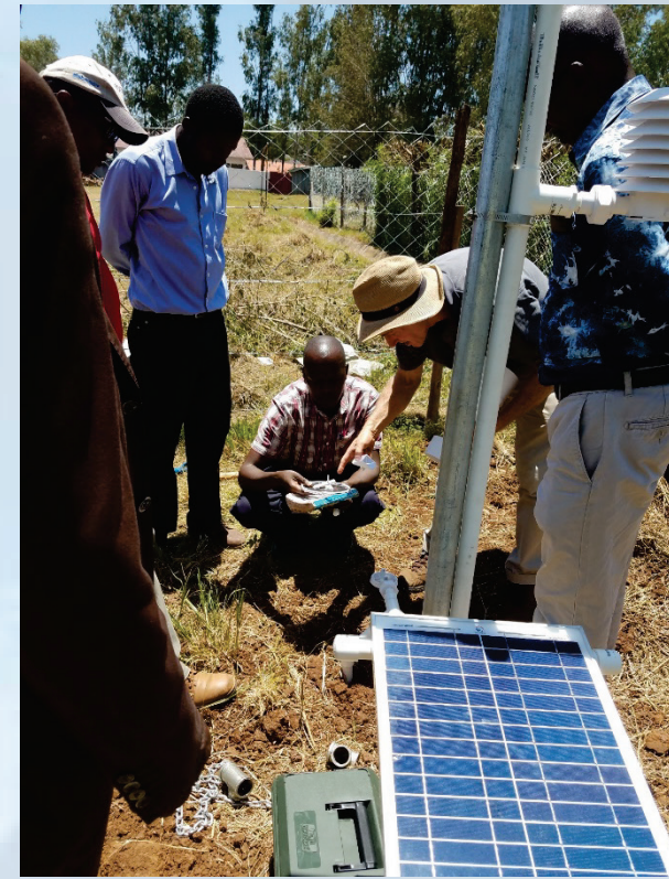
3D PAWS and Manual Precipitation Gauge Comparison
