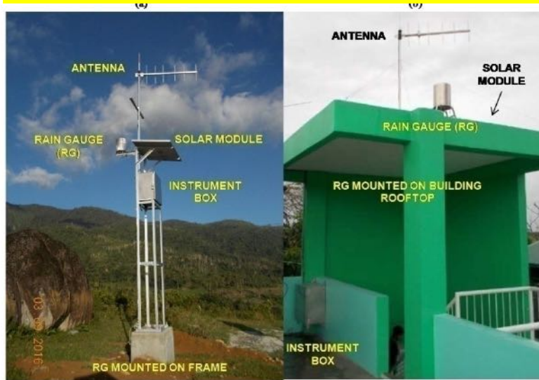
Fig. 4. Rain-gauge Installation (a) on frame and (b) on building rooftop.
