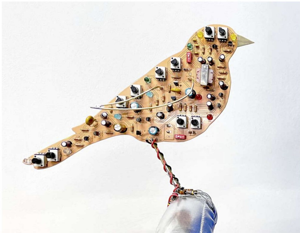
Image caption above: Kelly Heaton, "Printed Circuit Bird (Peach Bird)," 2020. Custom analog electronics and printed circuit board with a clear solder mask, which makes the copper appear peach-colored. 7" x 9" x 1.5" Image caption below: Kelly Heaton, "Schematic for Deep Fake Birdsong," 2020
